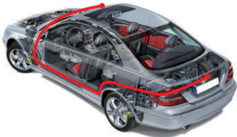
**Solution B:** install the rear view camera on the top of the rear windshield glass.
